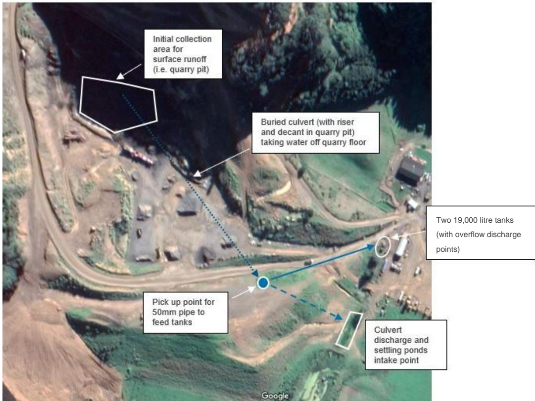
Figure 10. Water collection system
